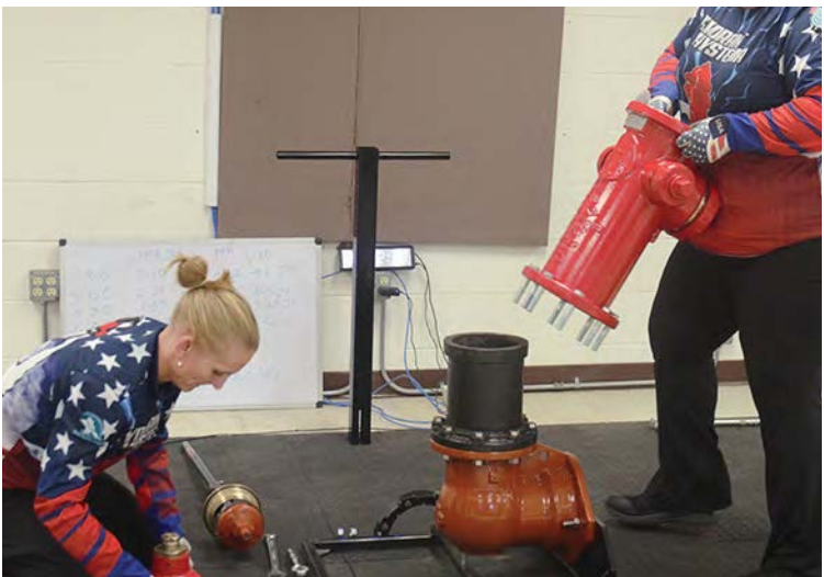
Angela lifts the main body of the fire hydrant into place while Katy works on affixing bolts to the bonnet (the top) of the hydrant.
